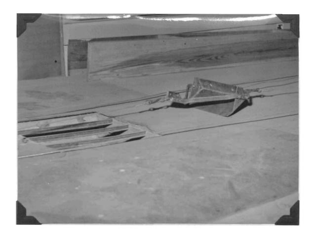
Figure 2. Photograph of Slope Bail Hoe Type Scraper with the blade bolted at a 45 degree angle to the line of pull.
