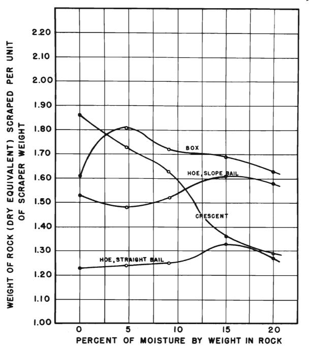
Figure 13. Relationship between equivalent dry weight of rock scraped and original moisture content of rock.
