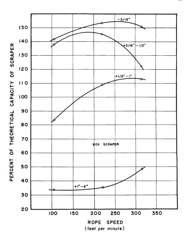
Figure 10. Relationship between box scraper capacity and rope speed with sized rock.
