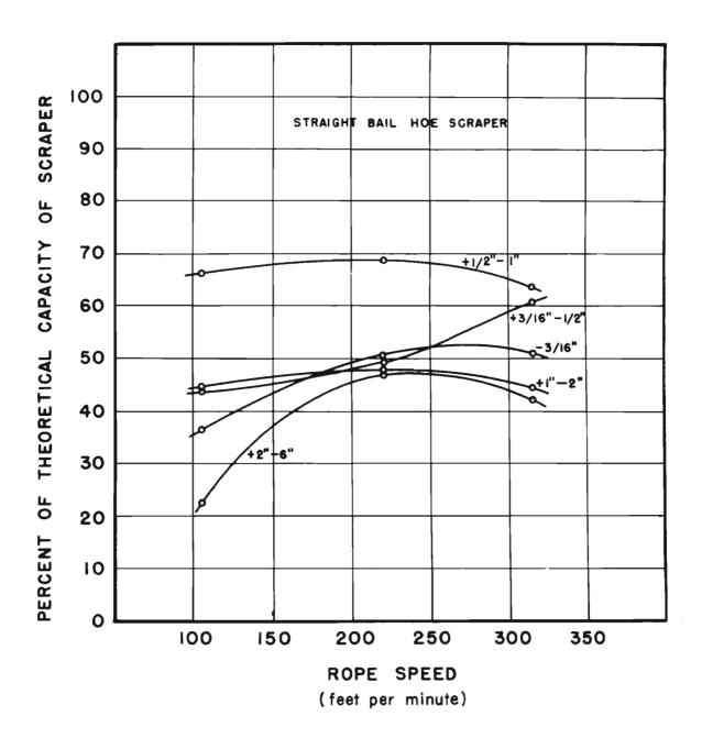
Figure 8 Relationship between straight bail hoe scraper capacity and rope speed with sized rock.
