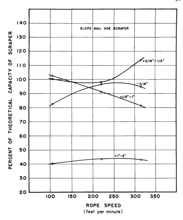
Figure 9 Relationship between slope bail hoe scraper capacity and rope speed with sized rock.
