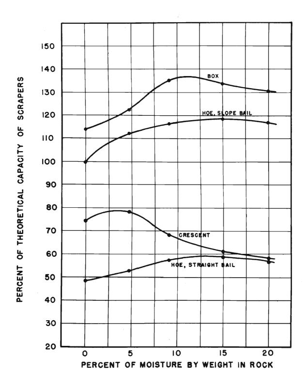
Figure 12. Relationship between scraper capacity and moisture content of rock.
