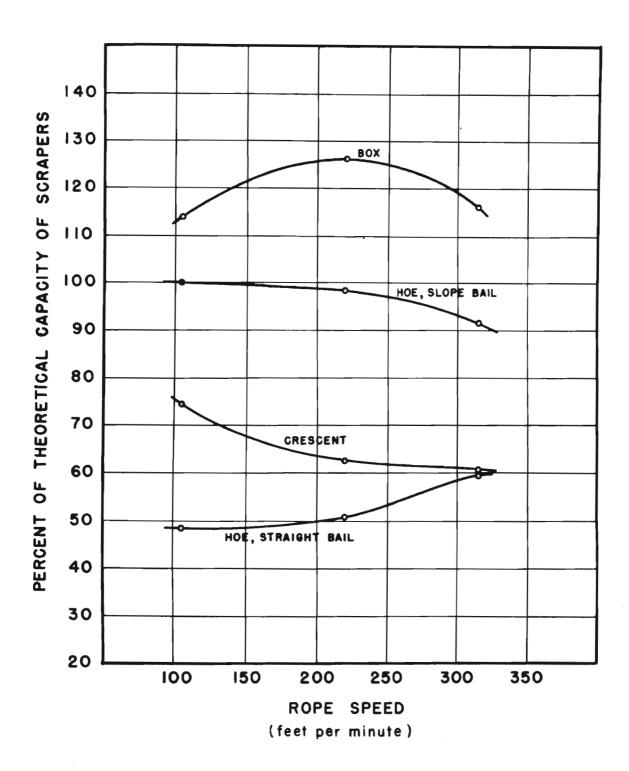
Figure 7. Relationship between scraper capacity and rope speed with mixed-size rock.
