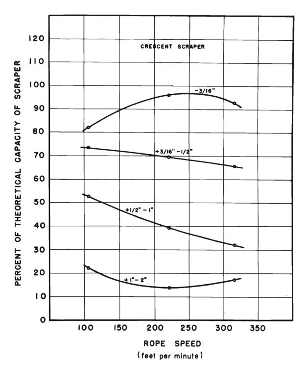
Figure 11.Relationship between crescent scraper capacity and rope speed with sized rock.
